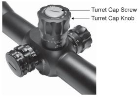
After your initial adjustments, fire another shot to make sure you are on target. Then move to your desired zero range and continue the process of adjusting the turrets to zero in the scope. Fire a three shot group and make any final adjustments based on the center of that group. To reset each turret knob to zero, remove the turret cap screw, pull off the turret cap knob, rotate the cap so the "0" will line up with the dot on the scope, push the knob back down, and replace the turret cap screw.
