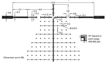
The BRS series scopes have a first focal plane reticle so the subtensions are accurate at any magnification.
