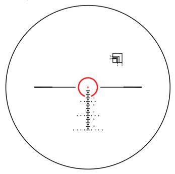
The Rugged 1-8x24 R-MIL is a second focal plane scope and must be set at the maximum magnification (8x) to accurately use the reticle for ranging and holdover.
